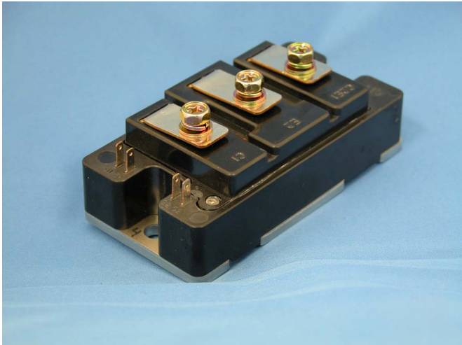
Fig. 1. External view of 1.2kV/100A, all-SiC Half H-Bridge power module.
