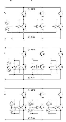
noise is minimized through the use of auxiliary emitters and local power supply decoupling capacitors. This circuit is suitable for use with modules rated up to about 200A. Figure 3.2C shows the recommended circuit for IGBT modules rated 300 amps or more. In this circuit separate isolated power supplies are used for each low side gate driver in order to eliminate ground loop problems.
