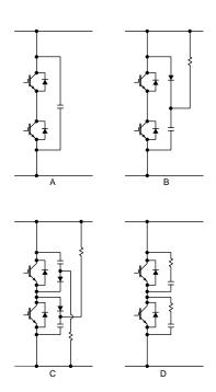
"C" of Figure 3.5. The initial voltage spike ( $\Delta V_1$ ) is caused by a combination of the parasitic inductance in the snubber circuit and the forward recovery of the snubber diode. If a fast IGBT snubber diode is used the majority of this spike will be due to the inductance of the snubber. In this case, we can compute the magnitude of  $\Delta V_1$  using Equation 3.1.
